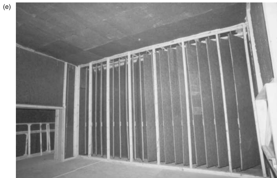
Figure A.1.9 ( continued ) (e) The 20-panel array in place during Measurement No 10.
